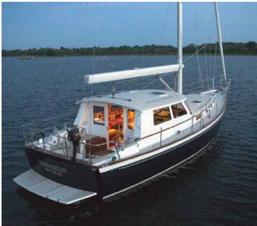
The raised doghouse and cockpit are on one level while the galley and cabins are down two steps going forward
